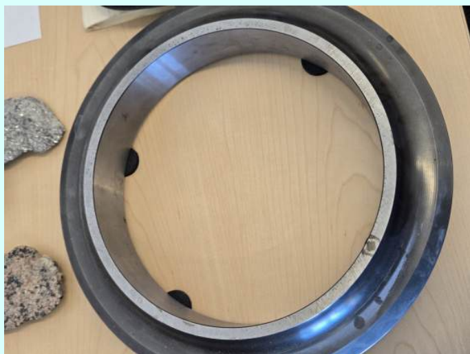
One of the multiple rings that do the cutting.
