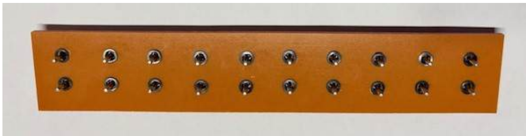
2mm Star Lock washers hold the connectors in place
