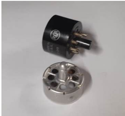
The removed octal base and the notches in the octal shell.
