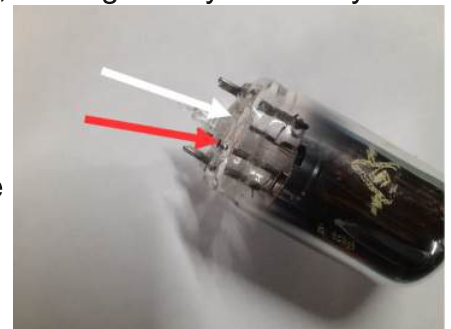
The white arrow above points to missing pin 4, the red arrow points to the nub that is pin 5 on the bare 3LF4.
