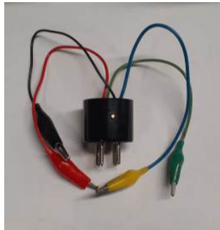
Adapter to test UV199 tube
