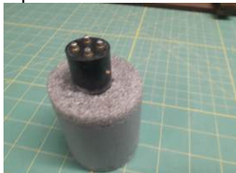
The tube holder for the UV199, 3Q5GT and 3LF4 tubes. It is held closed with duct tape.
