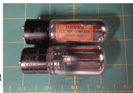
The top tube is a real UV199 tube, complete with a radio shop sticker from a shop in Lincoln, Nebraska. The bottom tube is a re-based 3LF4.
