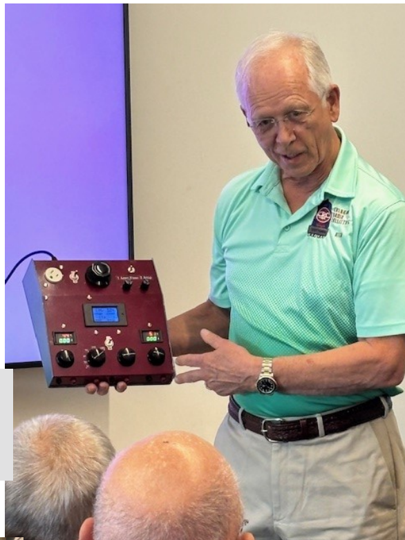
Rich Kuberski with another in his line of handmade power supplies (Volt-O-Matics). This one had an A/C outlet controlled by a variac
