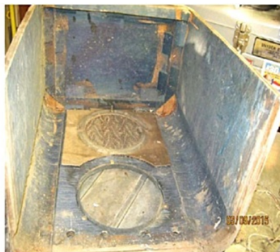
The plywood chassis board at the bottom was delaminated and detached from the visibly warped cabinet sides.
