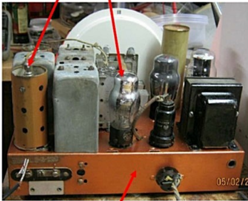
Cleaned and repainted chassis
