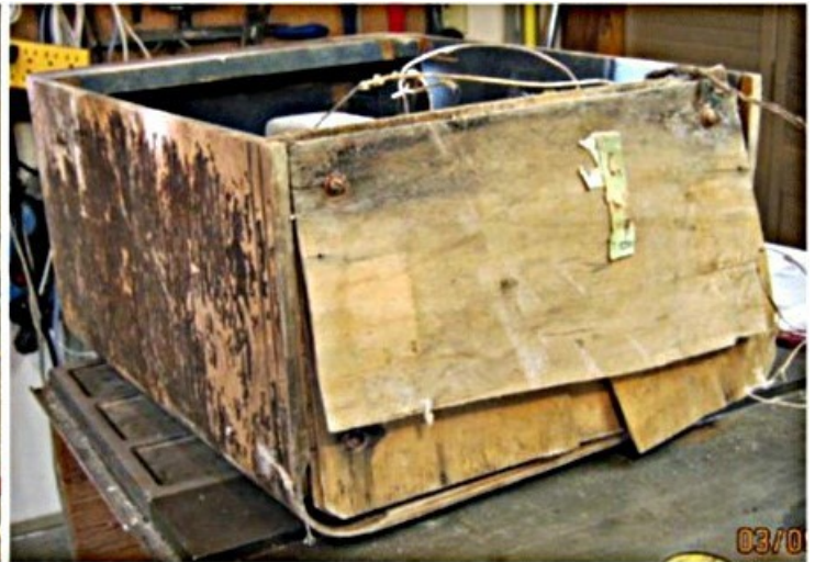
The artificial wood grain skin was in ruins from exposure to the weather, and the four knobs at bottom were missing.
