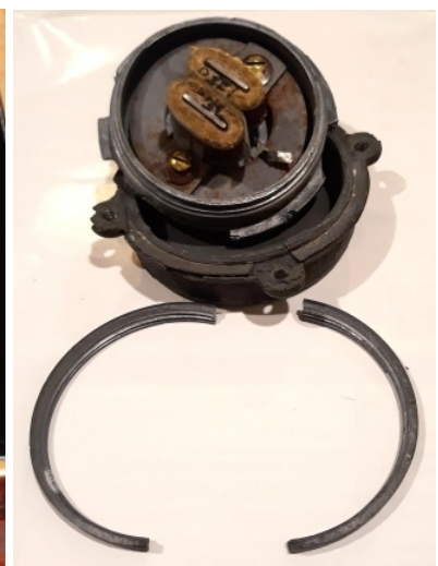
The housing & cap shown at the top with the broken-off threaded portions of the housing shown below
