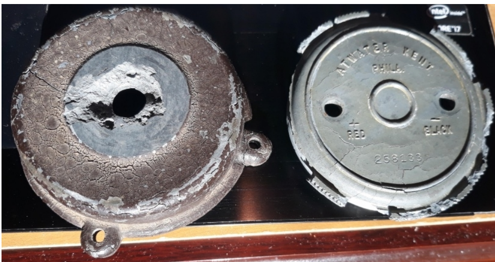
The output housing Cracked with the output pipe & mounting tab broken off
