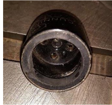
Centering strip is glued in the 01A base
