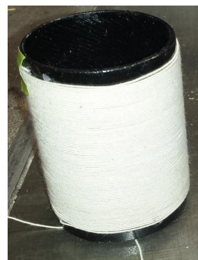
The secondary coil as wound
