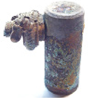
Figure 3: Steel Post With Partly Molten Brass Screw and Nut
