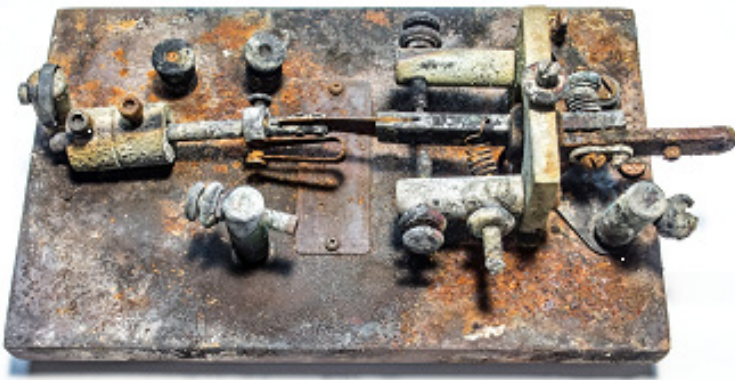
Figure 2: Telegraph Apparatus Key After the Fire
