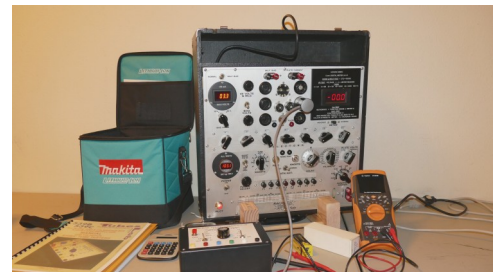
Bill Eccher talks about modifications he has made to this tube tester.
