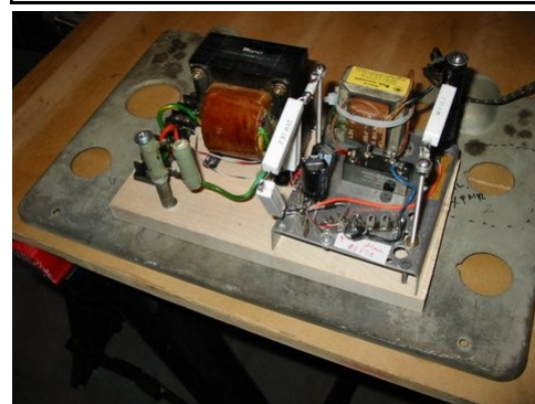
Photo #6 New Power Supply Sub-Chassis
