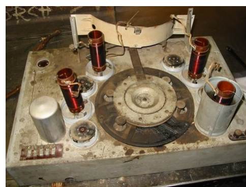
Photo #3 Original RE-57 Radio Chassis
