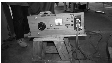
The control Panel for the Tesla Coil
