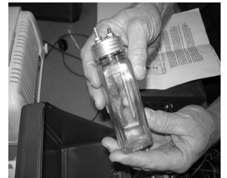
One of the four chemical rectifiers from the Philco battery eliminator
