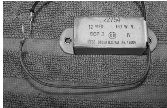
6. Box capacitor rebuilt
