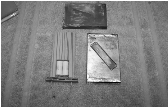
3. Filler with new capacitors in place, old capacitor at top
