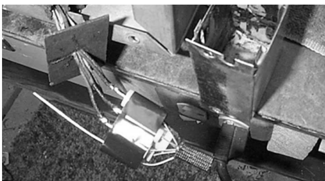
4. Metal can multi-section capacitor ready for reassembly
