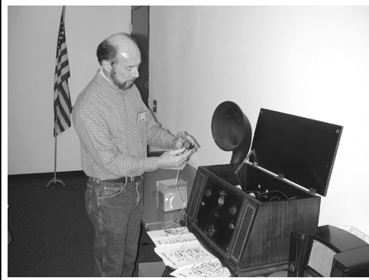
Tom Pouliot explains and demonstrates solid state tube replacements. The devices are wired onto dud tube pins and are completely hidden.
