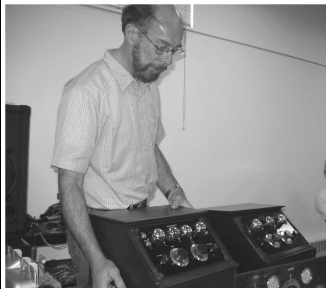
Tom Pouliot displays two very fine radios; A Colin B. Kennedy Co. model V 1923 (3 tube) and a model VI 1924 (4 tube) - both are battery operated radios.
