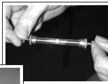
Don Andrus demonstrates and explains the operation of a Coherer detector. Don hand built the dectector, along with both the receiver and the spark transmitter.
