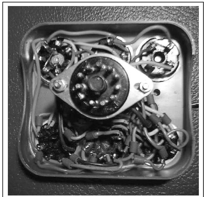
Underside of the interchangeable tube socket assembly
