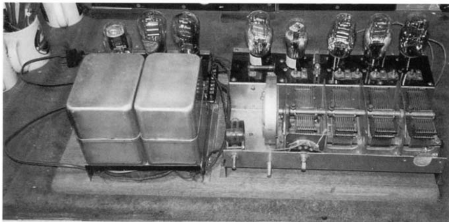
The completed power and audio chassis (L) with the completed RF/Detector chassis (R). New wiring and clean up required.
