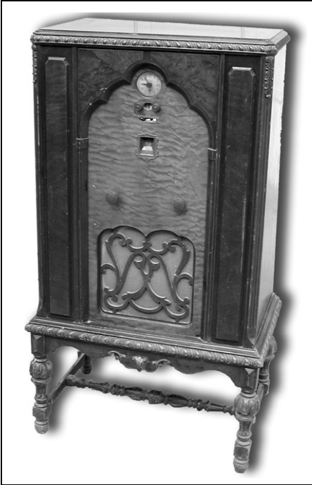
Silvertone model 112, 1930 clock controlled turn on/off and pre-set station tuning
