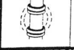
Bottom—No shield between coils in ordinary radio. Signals jump back and forth, making howl. Factory cuts resistor to cut howl—thus you miss many stations.
