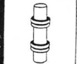
Bottom—2 section coils of ordinary radio. Mounted vertically. Wood dowel shrinks in dry climate—coils slip down. Expands in wet climate—compresses wires, causes short circuit.
