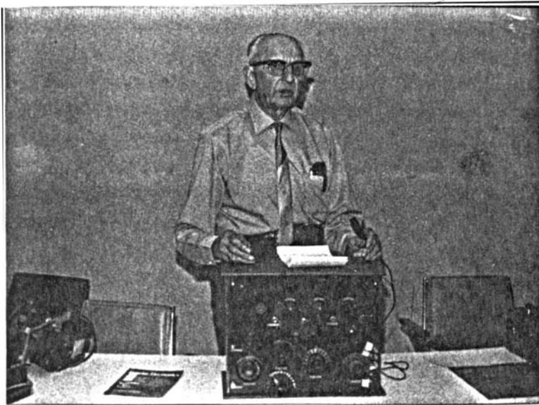
Emil Berndt and close up (below) of receiver he built using 3 WD-11 tubes.
